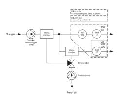
To extend the measuring range and protect the measuring cells against overloads, you can set thresholds which, when exceeded, activate sensor protection. Thresholds for a variety of parameters can be set, depending on the measuring cells that are connected.
