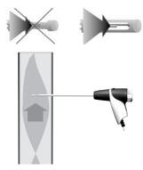
The thermocouple of the flue gas probe must not lie against the probe cage.
